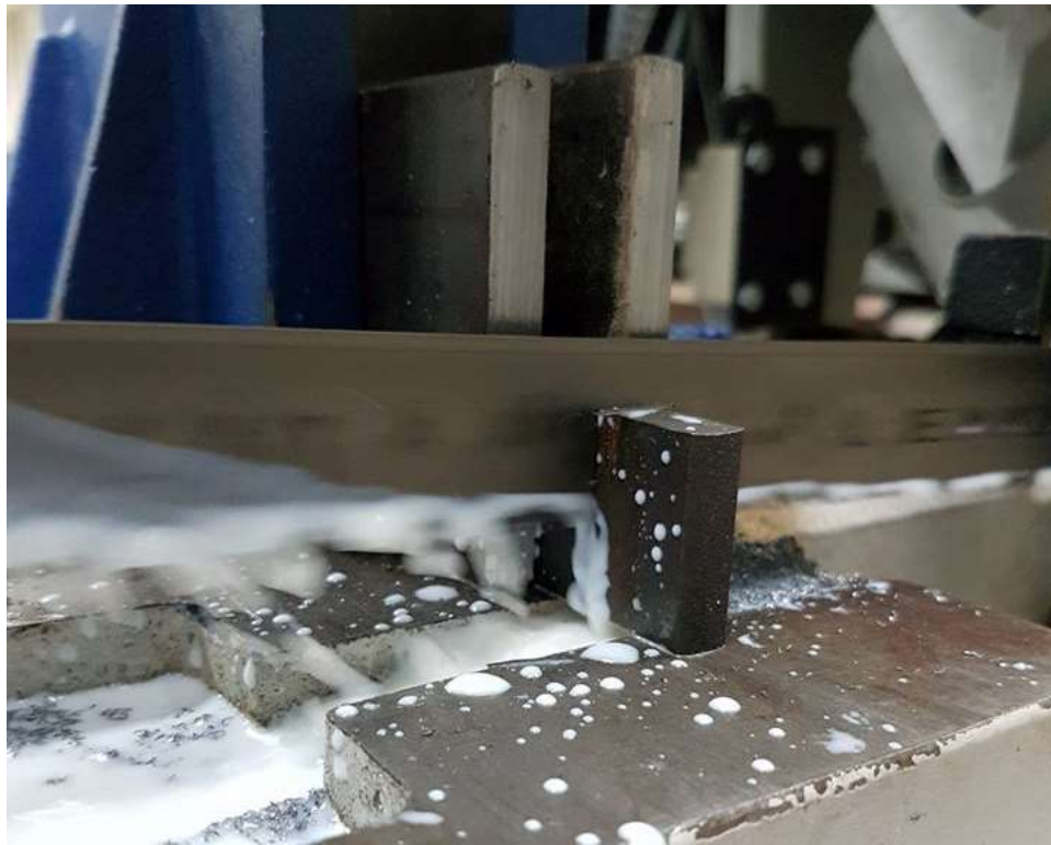
Figure 3.4 Cutting off the steel samples from bar stock by a horizontal band saw
