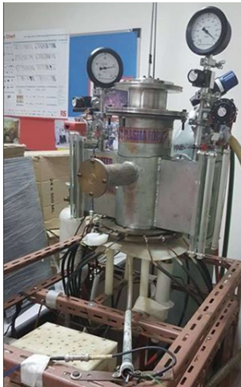
Figure 3.17 3 kJ Mather Type Dense Plasma Focus Device
