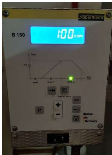
Figure 3.10 Time setting to maintain constant annealing temperature
